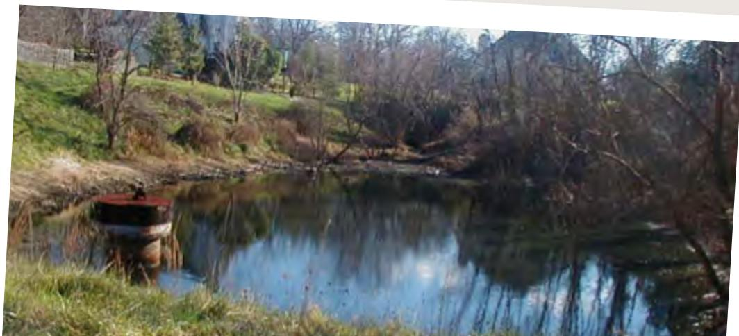
Figure 2. Typical stormwater management pond showing overflow riser.
